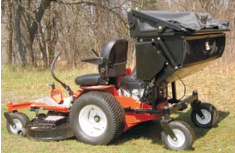
Conversion accessory converts the triple bag manual collector to a 9-bushel release from seat system.
